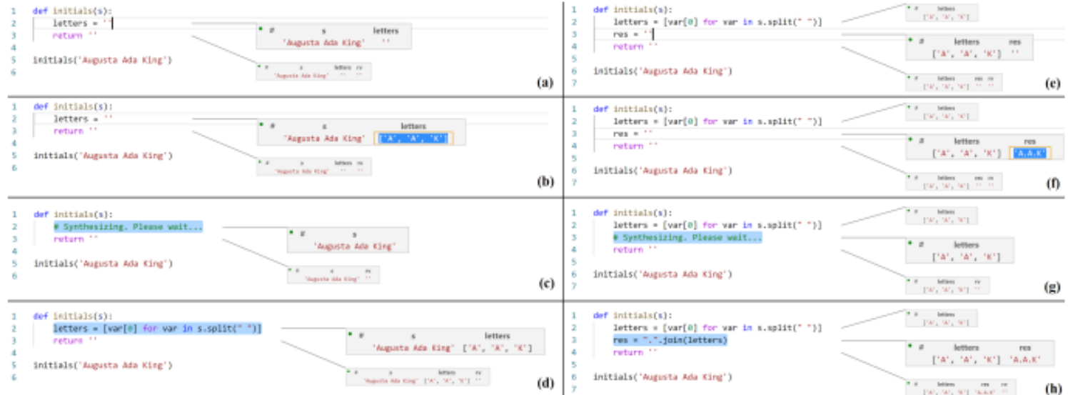
Figure 1. Writing code using SNIPPY: (a)-(d) generates the first statement and (e)-(h) generates the second statement.
